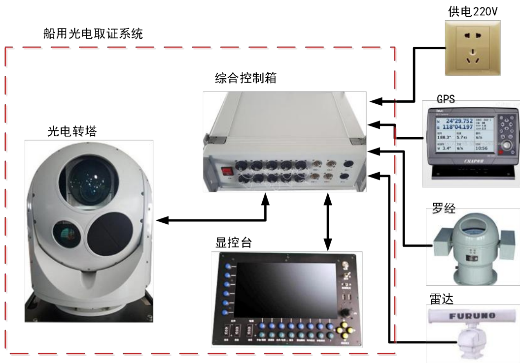
Fig. 1 Composition diagram of marine electro-optical turret system
