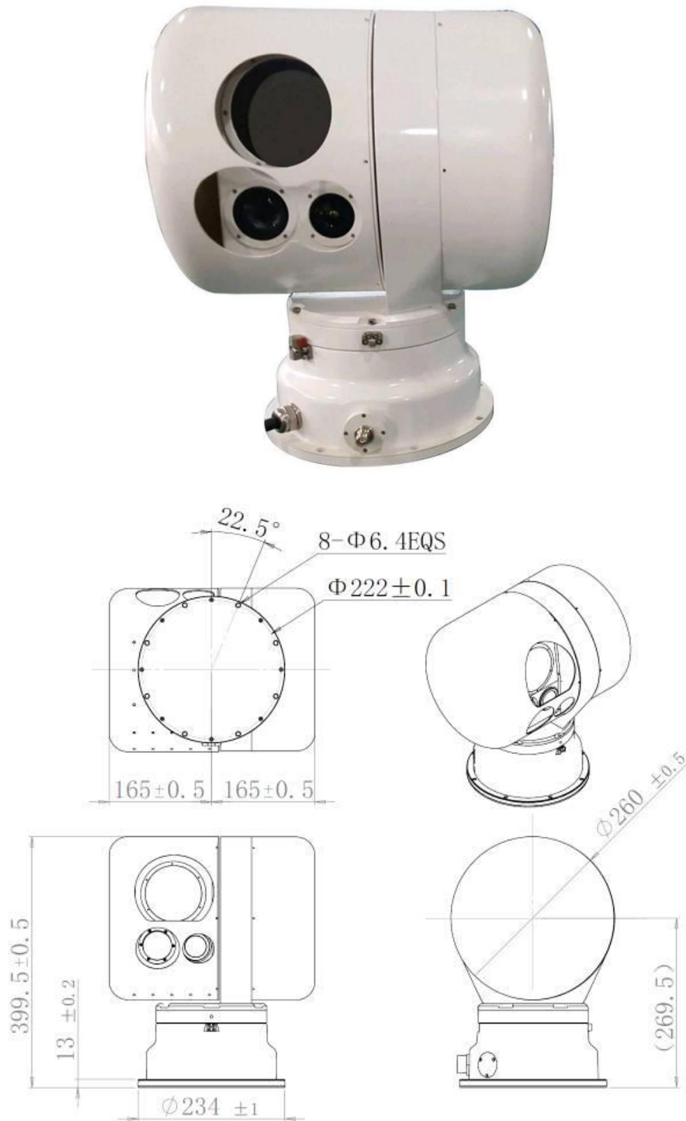
Fig. 2 Outline dimensions and installation interface diagram
