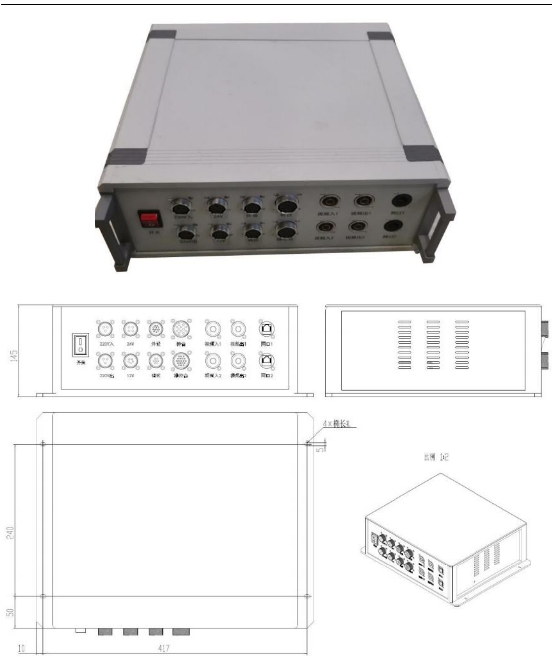
Fig. 4 Overall dimensions and installation interface diagram of integrated control box
