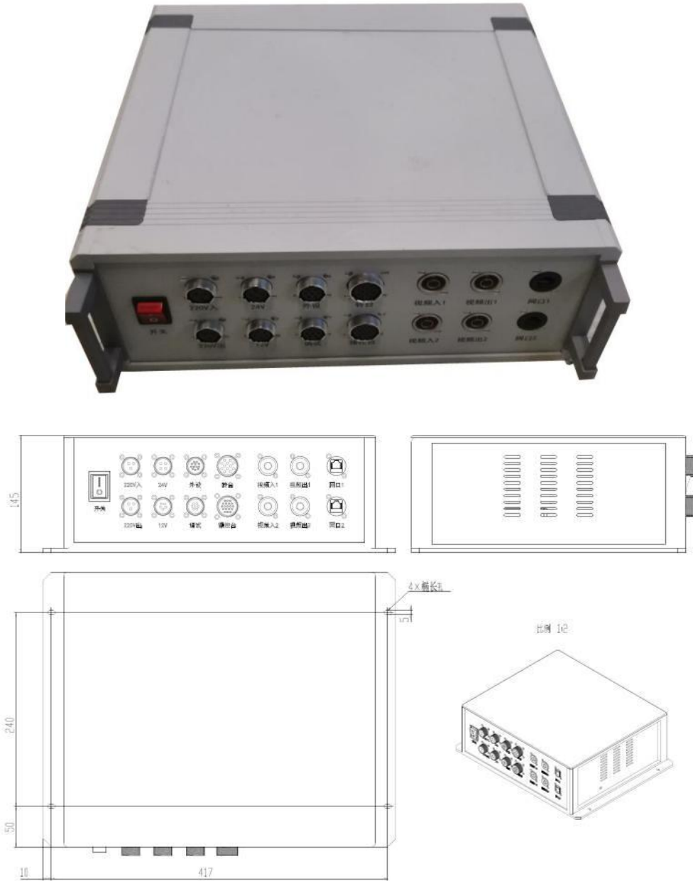
Fig. 4 Overall dimensions and installation interface diagram of integrated control box
